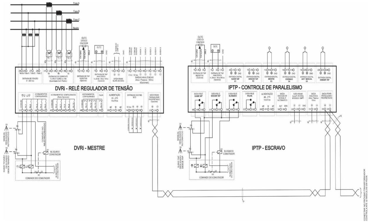
Figure 8 – DVR Master/IPTP Slave Link Diagram
