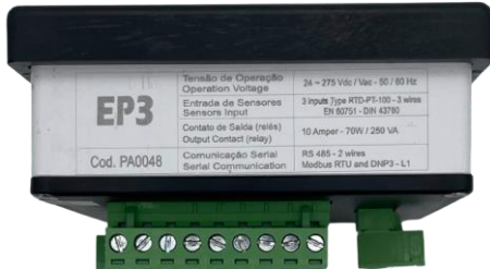
Figure 5 – Location of the technical data label.
