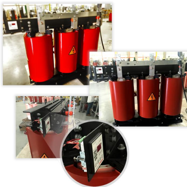
Figure 10 – EP3 installed in a medium-voltage dry-type transformer.
