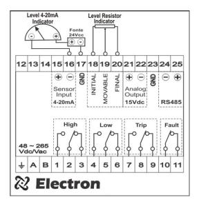
Figure 1 – Connection diagrams
