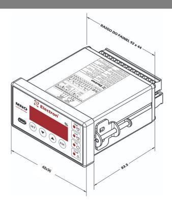
Note: Slot in the panel must be 92x44mm
