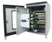
**Outdoor/Outdoor Double Door Panel:** Outdoor box with double door for mounting instruments, accessories and power transformer control and power wires. The external door contains a glass viewer with UV protection for viewing the quantities measured by the temperature monitor and the panel contains special paint that is resistant against weather and its degree of protection is IP 55, according to NBR IEC 60529:2017.
