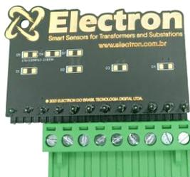
**PT-100 signal reference card:** This accessory was developed to verify the temperature value displayed by equipment with PT-100 3-wire RTD sensor input. It consists of precision resistors that send an equivalent fixed and constant resistance signal for selection between 3 different ranges, 0 °C (100 Ohms), 26 °C (110.9 Ohms) and 200 °C (175.86 Ohms).
