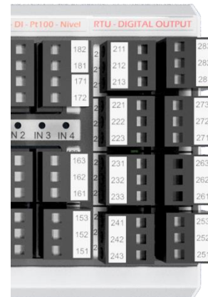
Figure 20 - Illustration of digital outputs module to SPDT NAF Relay
