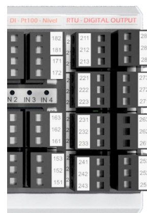
Figure 20 - Illustration of the module digital outputs to SPDT NAF Relay
