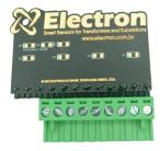
**PT-100 Signal Reference Card:** This accessory was developed to verify the temperature value displayed by equipment with PT-100 3-wire RTD sensor input. It consists of precision resistors that send a fixed and constant equivalent resistance signal for selection between 3 different ranges, 0 °C (100 Ohms), 26 °C (110.9 Ohms) and 200 °C (175.86 Ohms).
