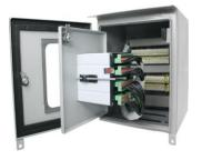
**Double Door Panel for Outdoor/Outdoor Use:** Box for external use with double door for mounting instruments, accessories and passing control and power wires of the power transformer. The external door contains a glass display with UV protection for viewing the quantities measured by the temperature monitor and the panel contains special paint that is weather resistant and its degree of protection is IP 55, as per NBR IEC 60529:2017.
