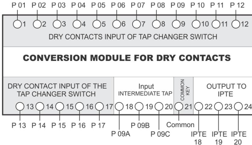
**\* This module must be used when the switch crown is made of dry contacts, without resistors.**
