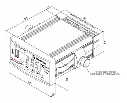
Figure 2 - Illustration of Monitemp Dimensions
