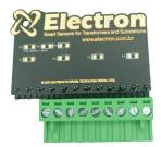
**Reference card for PT-100 signal:** This accessory was developed to perform the verification of the temperature value displayed by equipment with input of RTD PT-100 sensors of 3 wires. It consists of precision resistors that send an equivalent fixed and constant resistance signal for selection between 3 different ranges, 0 °C (100 Ohms), 26 °C (110.9 Ohms) and 200 °C (175.86 Ohms).
