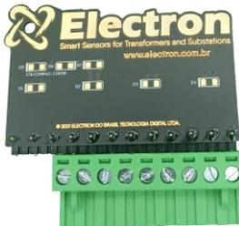
**Reference card for PT-100 signal:** This accessory was developed to perform the verification of the temperature value displayed by equipment with input of RTD PT-100 sensors of 3 wires. It consists of precision resistors that send an equivalent fixed and constant resistance signal for selection between 3 different ranges, 0 °C (100 Ohms), 26 °C (110.9 Ohms) and 200 °C (175.86 Ohms).
