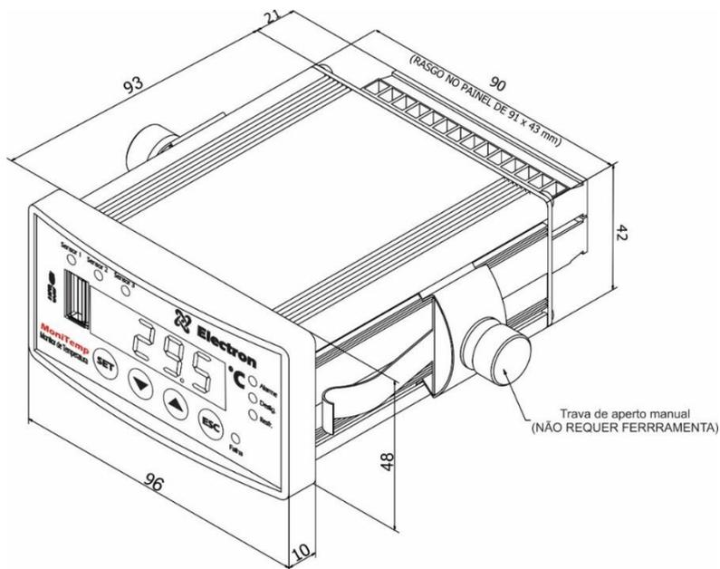
Figure 2 - Illustration of MoniTemp Dimensions
